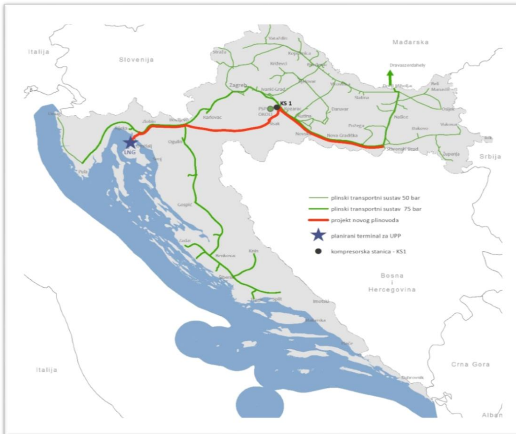
Figure 3 The existing transmission system of Plinacro, location of the LNG terminal, CS 1 and Omišalj-Zlobin-Bosiljevo-Sisak-Kozarac-Slobodnica gas pipeline
